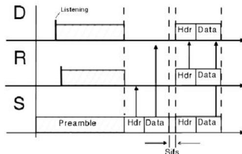
Figure 2 - Frame sending sequence between a source S, a relay R and a destination D
