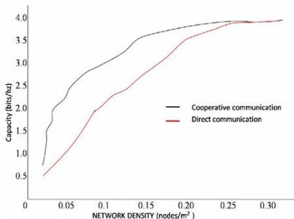
Figure 4 -Capacity as function of the nodes density
