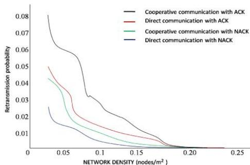
Figure 3 - Retransmissions probability as function of the nodes density
